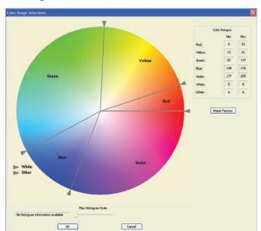
ColorCount software allows you to define the colors you want to count. QCount comes programmed with seven preset colors including "white" and a user-definable color. This allows for fast startup and use right out of the box. Users also have the flexibility to easily define their own color settings with no limitations — defining individual colors or even a range of shades as one color.
