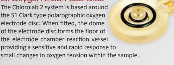
The electrode disc comprises a central platinum cathode and a concentric silver anode. Preparation includes the addition of electrolyte and the application of a thin oxygen permeable P.T.F.E. membrane to the electrode dome. Once prepared and positioned in the electrode chamber, the disc is connected to the Oxylab control circuitry which applies a small polarising voltage between the electrodes. In the presence of oxygen, a small current is generated proportional to oxygen activity in the sample.
