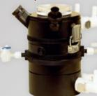
The LD2/3 leaf-disc electrode chamber allows oxygen uptake / evolution measurements to be performed from leaf-discs, excised needles, algae, mosses, lichens etc with a surface area of up to 10cm<sup>2</sup>. A prepared S1 oxygen electrode disc is mounted directly below the sample chamber with the dome of the electrode forming
