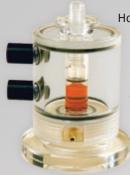
However, due to the gas-tight plunger assembly, the DW1/AD lends itself particularly well to respiration assays in small sample volumes where any minute diffusion of ambient oxygen into the chamber may cause measurement artefacts. The DW1/AD oxygen electrode chamber is constructed from clear cast acrylic providing good sample visibility & uniform illumination.
