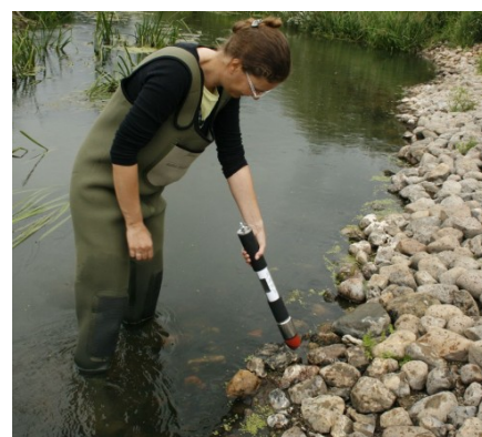
BenthoTorch used in the AQUAREHAB project in Denmark and Belgium
